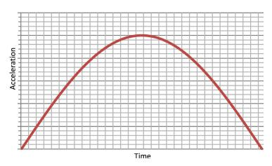
ShockWatch impact indicator shock response curves are based on a half-sine shock pulse (shown above). A time, acceleration point on the half-sine curve can be correlated to the same point on the impact indicator activation response curves.
